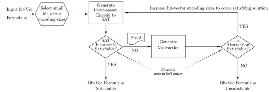
**Fig. 1.** Abstraction-based approach to solving bit-vector arithmetic
